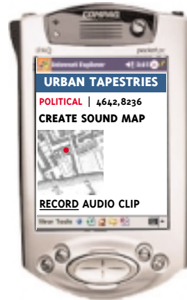
User prompted to record audio clip for sound maps .WAV file linked to GSM / GPS / WiFi reference
